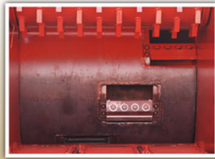
Drum Morbark's proven drum with staggered knife pattern and carbide edged knife holder.
