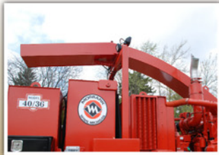
Discharge Directional flow discharge chute is hydraulically adjustable by remote control for maximum chips loads.
