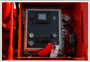
Morbark Integrated Control Systems The ultimate diagnostic system; monitors hydraulic pressures, temperatures, clutch systems and engine efficiency while automatically adjusting to maximize performance.
